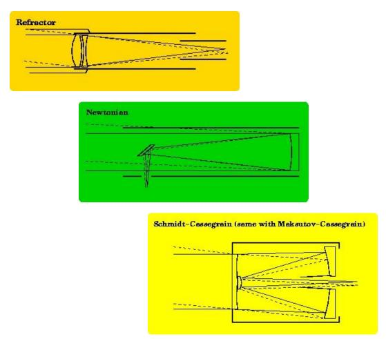
Top: In a refractor, a lens system focuses the light.
